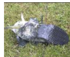
BCBI Boot after 70g explosion on heel
