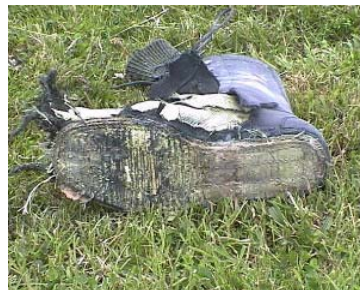
BCBI Boot after 50g explosion on ball
