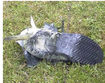
BCBI Boot after 70g explosion on heel
